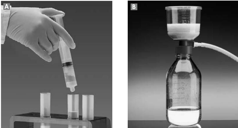
**Figure 2** **A** The syringe-format QIAfilter Maxi Cartridge in use with QIAGEN-tips in the QIARack.
